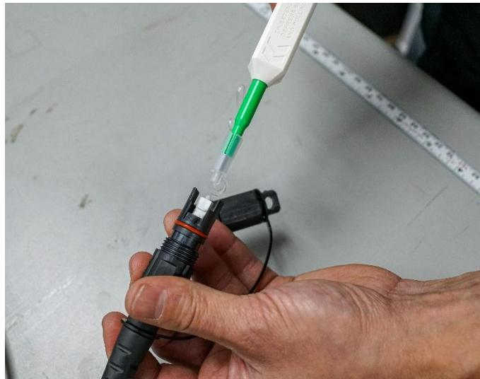
3.5 Replace the dust cap until the connector until is ready for use
