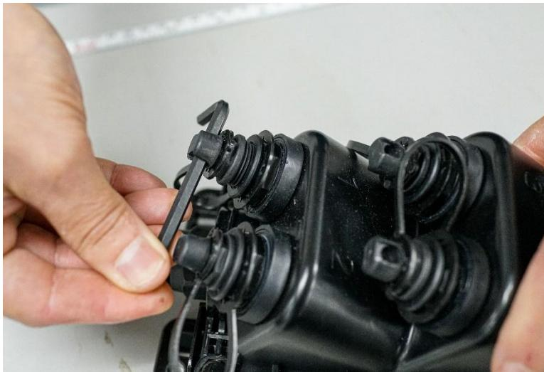
4.4 Inspect the end face of the connector by using a visual scope following the Manufacturer's instructions., ref 3.3 image.
