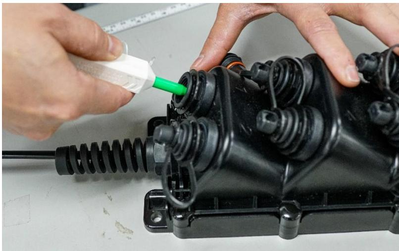
4.6 When the adapter is clean install the drop cable and tighten.
